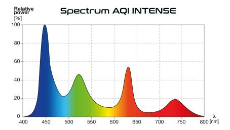
UNIQUE SPECTRUM INTENSE series lamps produce vivid colours and their spectral emission is characteristic for so called RGB lamps. What is unique and innovative on this RGB aquarium light is the broadening of spectrum with deep and far red. This allows for the appropriate activation of fytochromes both in Pr and Pfr stage. Far red light deeply penetrates plant tissue allowing shaded parts of plants to photosynthesize too.
